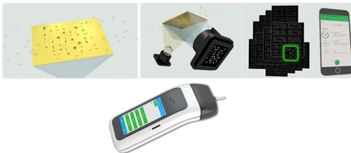
Fig. 1.: Neose device developed by Aryballe with above from left to right, the 3 key steps of the measurement: Binding of VOCs (or odorous compounds) on the biosensors arrayed on SPR prism covered by a gold layer ; interrogating the surface with O-cell based on SPRi ; Data Treatment: image analysis and data transfer
